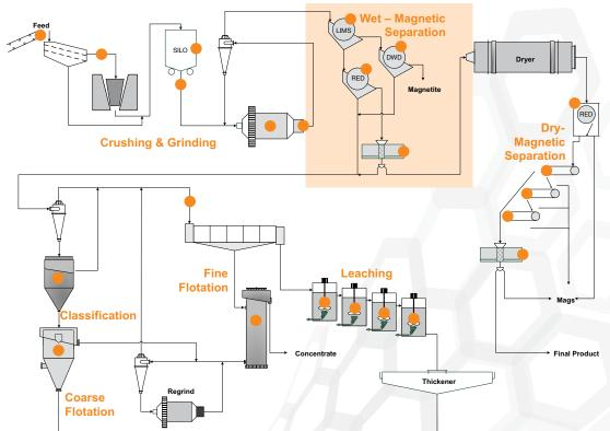
Whether it's processing high volumes of iron ore, or removing micron-sized ferrous or paramagnetic contaminants from valuable minerals, Eriez offers a complete range of continuous and batch magnetic solutions for wet processing. In hard rock mining, specialized magnetic equipment improves ball mill efficiencies by removing worn steel media fragments or using them as a protective liner.
