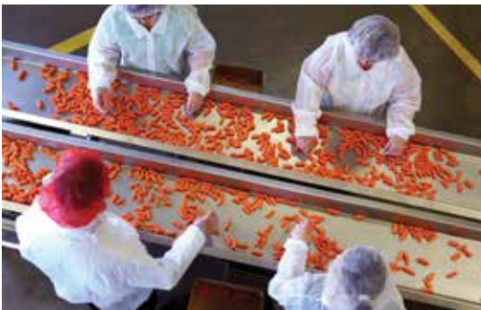
Sanitary vibratory conveyors move carrots past inspectors in a food packaging plant
