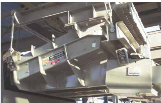
A heavy-duty feeder meters material to a magnetic drum in an iron ore mine
