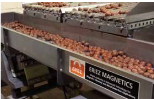
A combination screener and feeder moves chocolate candies into a wrapping operation
